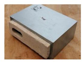
**1. For inclusion in brick or stone walls.** The front of the nest chamber is faced with a slip made of brick, stone or cast in a 50:50 mixture of sharp sand and cement. The face of the nest chamber is scored and has small holes for glue to penetrate. The glue used is Fixall maximum strength. This configuration is suitable for both new build and for retrofit.
